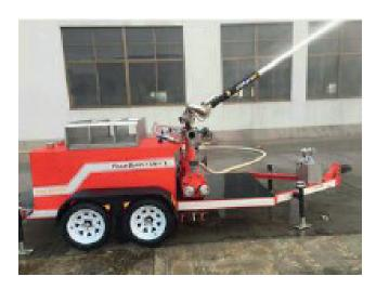
With 1000L foam tank on the truck, and with fire monitor Specification:
